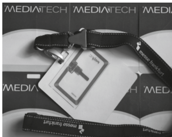
Fig. 8 Radio-frequency transponder with printed organic chip [20] used in a field trial at the MEDIA-TECH Expo conference 2008
